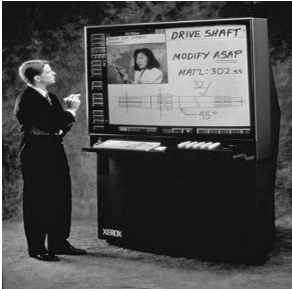
FIGURE 5 A commercial version of the Liveboard, sold by Liveworks in the mid-1990s, which evolved out of the original wooden laboratory prototype developed at PARC (Photo courtesy of PARC, Inc., http://www.parc.com )
